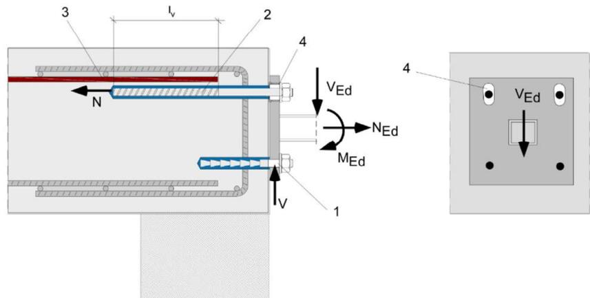
The required transverse reinforcement acc. to EN 1992-1-1:2004+AC:2010 is not shown in the figures. **The fischer rebar anchor may be only used for axial tensile force.** The tensile force must be transferred by lap to the existing reinforcement of the building. The transfer of the shear force has to be ensured by suitable measures, e.g. by means of shear force or anchors with European Technical Assessment (ETA).
