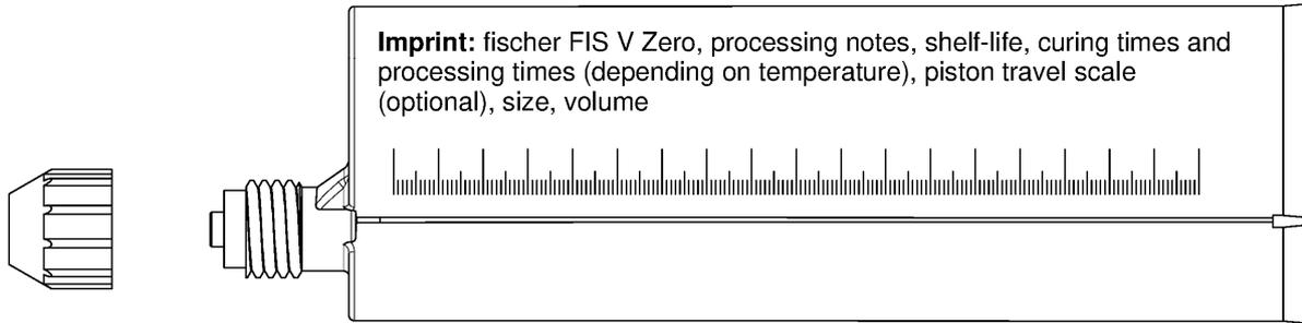
**Injection cartridge (coaxial cartridge) FIS V Zero with sealing cap; Sizes: 300 ml, 380 ml, 400 ml, 410 ml**
