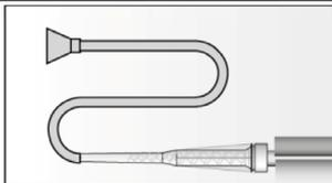
Assemble mixing nozzle FIS MR Plus or FIS JMR, extension tube and appropriate injection adapter (see **table B6.2**)
