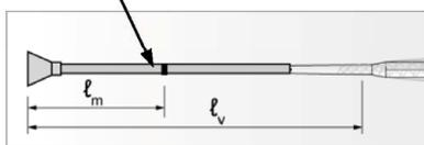
Mark the required mortar level  $l_m$  and embedment depth  $l_v$  resp.  $l_{e,ges}$  with tape or marker on the injection extension tube.
