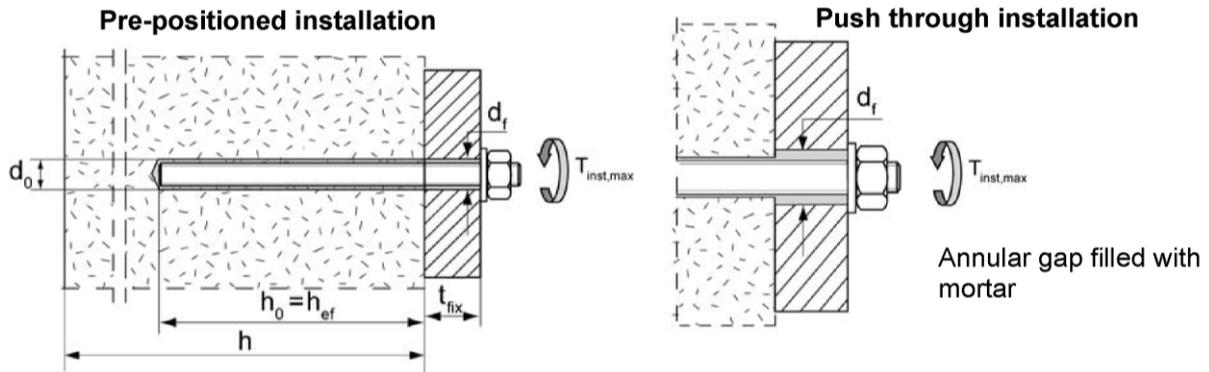
**Internal threaded anchors FIS E without perforated sleeve FIS H K; Installation in solid brick masonry and autoclaved aerated concrete**
