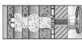
Mounting the fixture. $T_{inst,max}$ see Table B1.3                                                                                                                                                              |                                                                                                                                                                                                                                                        |
