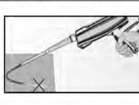
Press out approximately 10 cm of material until the mortar is permanently grey in colour. Mortar which is not grey in colour will not cure and must be disposed off |
