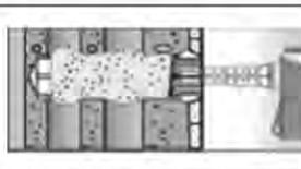
Fill the perforated sleeve completely with mortar beginning from the bottom of the hole <sup>1)</sup> .                                                            |
