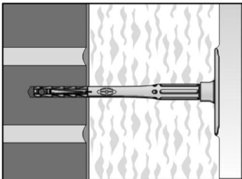
1. Drill the bore hole by the parameters acc. to Table B2.1 and the corresponding drilling method acc. to Annex C1.
