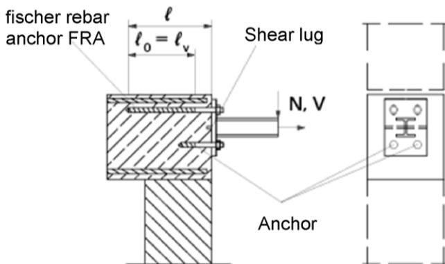
**Figure A8:** Lap of the anchoring of cantilevered buildings. In the anchor plate, the drill holes for the rebar anchors have to be designed as elongated holes with axial direction to the shear load.
