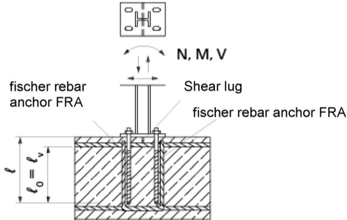
**Figure A6:** Lap to a foundation of a column under bending.
