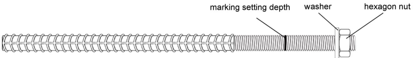
**Reinforcing bar (rebar)  $\phi$  8,  $\phi$  10,  $\phi$  12,  $\phi$  14,  $\phi$  16,  $\phi$  20,  $\phi$  25,  $\phi$  28,  $\phi$  32**
