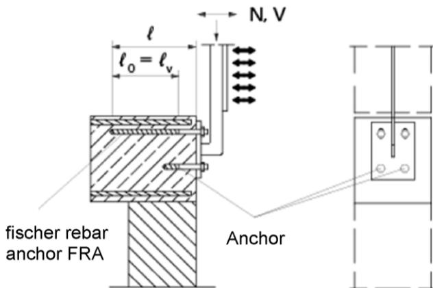
**Figure A7:** Lap of the anchoring of guardrail posts. In the anchor plate, the drill holes for the rebar anchors have to be designed as elongated holes with axial direction to the shear force.
