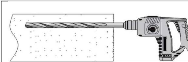
Drill hole to the required embedment depth using a hammer-drill with carbide drill bit set in rotation hammer mode or a compressed air drill.
