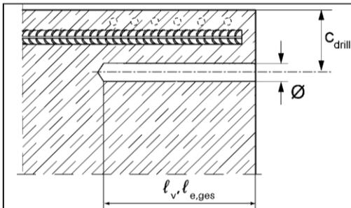
Measure and control concrete cover  $c$
