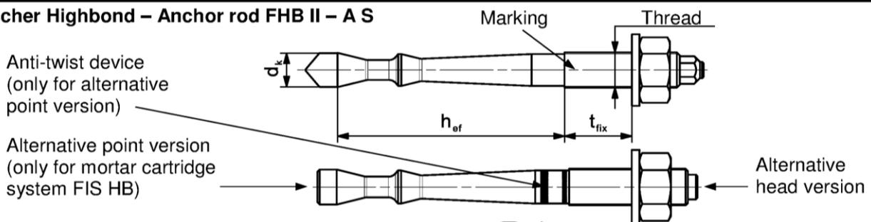
**Marking:** work symbol, size of anchor, setting depth. e.g.: M10x75
