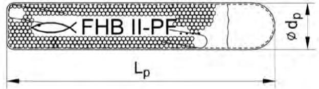
**Imprint:** work symbol, marking, anchor size and effective anchorage depth.
