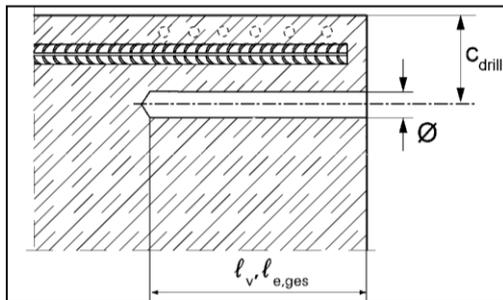
Measure and control concrete cover  $c$
