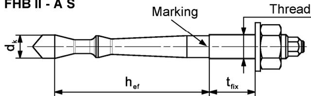
**Marking:** work symbol, thread diameter, embedment depth e.g.: M16x95
