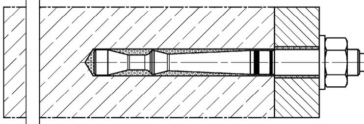
Pre-positioned or push through installation with subsequently injected fischer filling disc
