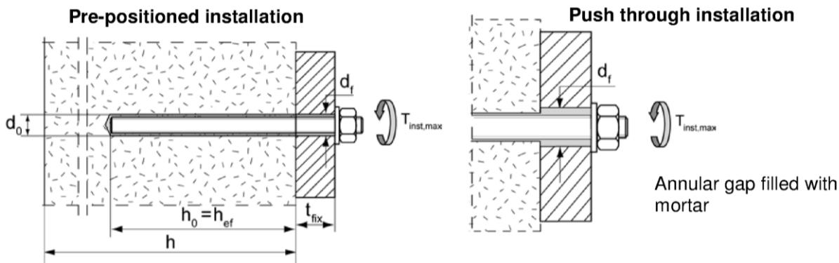
Internal threaded anchors FIS E without perforated sleeve FIS H K; Installation in solid brick masonry and autoclaved aerated concrete
