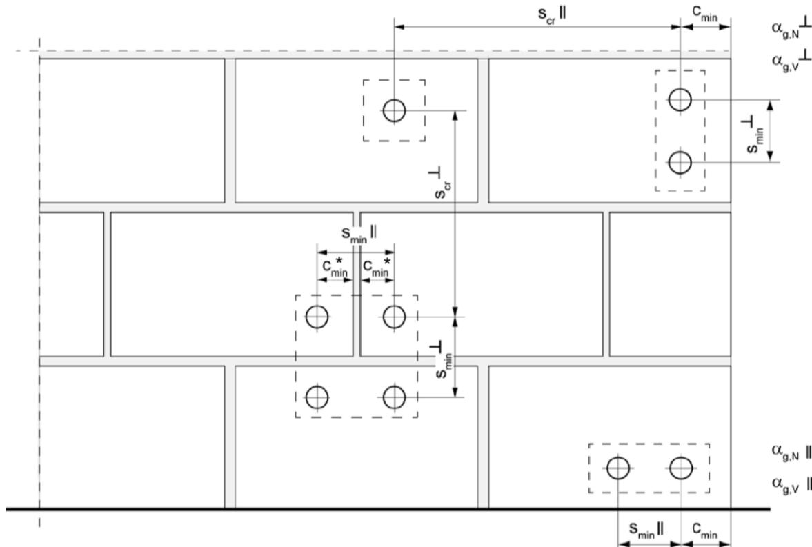
\* Only, if joints are visible and vertical joints are not filled with mortar
