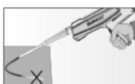
Press out approximately 10 cm of material until the mortar is permanently grey in colour. Mortar which is not grey in colour will not cure and must be disposed off                                                |
