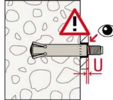
**5.:** The anchor is correctly expanded if the colour marking on the thread of the tapered bolt is visible.
