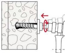
2.: Once the FZUB depth stop meets the concrete, create the drill hole undercut by making circular swiveling movements with the hammer drill while the hammer mechanism is engaged. Press the hammer drill firmly against the anchor base: 1 - 2 swiveling movements are sufficient for  $\varnothing 14$  mm, with 3 - 5 movements for  $\varnothing 18$  mm and  $\varnothing 22$  mm.
