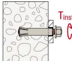
**6.:** Mount installation object (e.g. anchor plate), washer and nut and apply installation torque with torque spanner.
