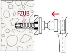
**1.:** Create a drill hole through the installation object perpendicular to the surface of the anchor base with a hammer drill, using the corresponding Zykon universal drill bit FZUB. The required drill depth is reached once the FZUB depth stop meets the fixture.
