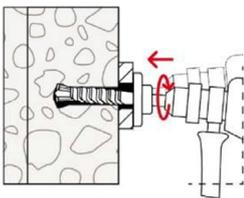
**2.:** Once the FZUB depth stop meets the fixture, create the drill hole undercut by making circular swiveling movements with the hammer drill while the hammer mechanism is engaged. Press the hammer drill firmly against the anchor base: 1 - 2 swiveling movements are sufficient for  $\varnothing$  14 mm, with 3 - 5 movements for  $\varnothing$  18 mm and  $\varnothing$  22 mm.
