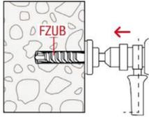
1.: The drill hole must be drilled at right angles ( $\pm 5^\circ$ ) to the surface of the anchor base with a hammer drill using the corresponding ZYKON FZUB drill bit. The required drilling depth is reached when the depth stop of the FZUB is in contact with the concrete.
