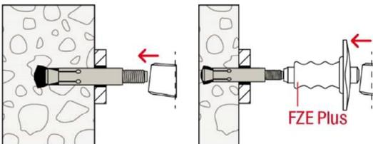
**4.:** Insert the anchor into the drill hole through the installation object (e.g. anchor plate) and then drive the expansion sleeve in with hammer-set device FZE Plus, using a manual hammer.
