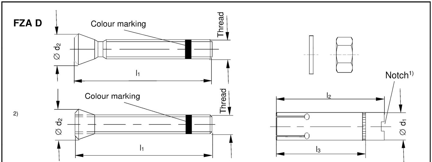
**Table A5.1: Dimensions through bolt anchor FZA D [mm]**
