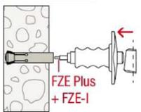
4.: Insert the anchor into the drill hole and then drive the expansion sleeve in with hammer-set device FZE Plus, using a manual hammer.
