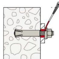
**Optional:** The gap between bolt and fixture may be filled with mortar (compressive strength  $\geq 50$  N/mm<sup>2</sup> e.g. FIS SB) after step 6 (for eliminating the annular gap). The filling disc is additional to the standard washer. The thickness of the filling disc must be considered for definition of  $t_{fix}$ . Countersunk of the filling disc in direction to the anchor plate.
