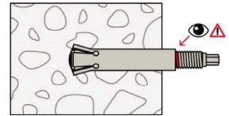
5.: The anchor is correctly expanded if the colour marking on the thread of the tapered bolt is visible or the gap  $u$  between conical bolt with internal thread and expansion sleeve (FZA I) is fulfilled. When using the FZA 12x40 ST the knurling on the sleeve is flush or below the concrete surface.
