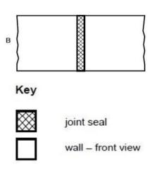
B tested vertical linear joint in a vertical test construction, and direct field of application according to EN 1366-4:2006 Table 1 and figure
