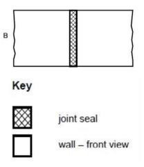
B tested vertical linear joint in a vertical test construction, and direct field of application according to EN 1366-4:2006 Table 1 and
