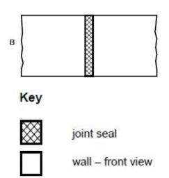
B tested vertical linear joint in a vertical test construction, and direct field of application according to EN 1366-4:2006 Table 1 and figure 12
