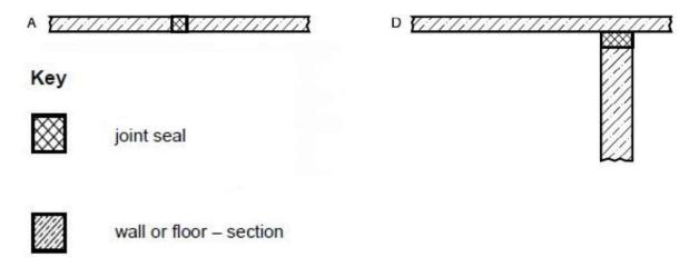
A tested linear joint in a horizontal test construction.
