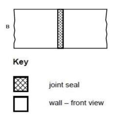
B tested vertical linear joint in a vertical test construction, and direct field of application according to EN 1366-4:2006 Table 1 and figure 12
