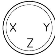
Marking at **X**: "O" for  $h_{ef} = 25$  mm
