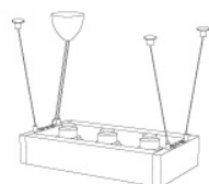
Single wire suspensions Order: 1 x Mech/Elec 3 x Mech only
