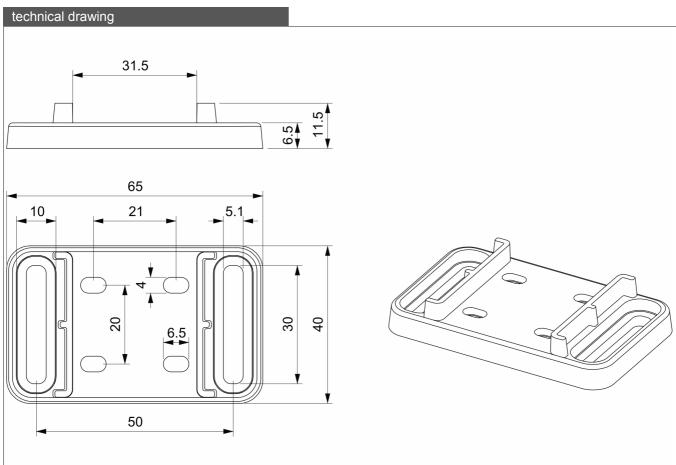
Plastic support for a fast installation and a simple positioning of our FC series door limit switch.
