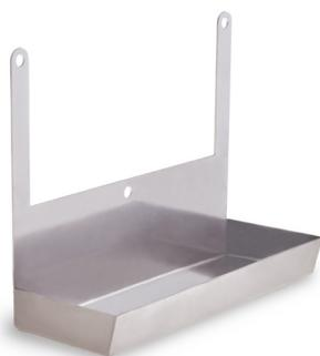
Drip tray is a stainless steel accessory to be positioned under the thermoelectric unit. It is used to collect the condensate generate on the cold heat sink inside the enclosure. Suitable for vertical installation.
