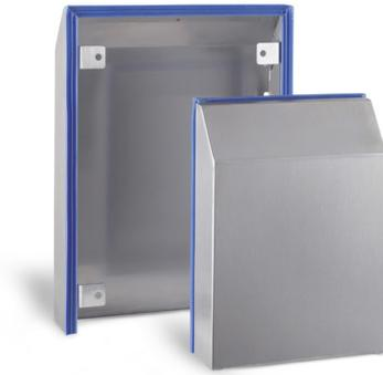
A protective cover for exhaust filters and filter fans in stainless steel (AISI 304) and UL Type 4X version equipped with a FDA-compliant silicone gasket for a safe use in food industry or outdoors. It effectively safeguards against rain, water jets and foreign particles by securely sealing the ventilation openings, by increasing the protection class to IP56. Available also in powder coated RAL 7035, UL Type 4.
