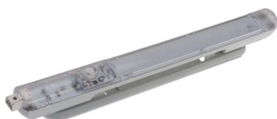
Thanks to a good color rendering, the FLL series LED lamps represent an efficient solution for enclosure lighting. Available in AC, DC or multi voltage versions and with ON/OFF switch or PIR sensor. FLL series offers the advantages of a swiveling system to direct light beam, optional magnetic fastening and a quick connection by screwless wiring system.
