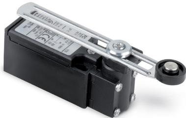
The limit switches ensure safety during maintenance work inside the electrical panels. They are applied on the frame of the cabinet and can turn on the lights, turn off a fan or a heater or cut off the power supply in general when the door is opened or closed.
