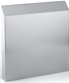
A protective cover for exhaust filters and filter fans in stainless steel (AISI 304) to safeguard against rain, water jets and foreign particles, by increasing the protection class to IP56. Available also in powder coated RAL 7035, UL Type 12 and in UL Type 4X version equipped with a FDA-compliant silicone gasket.
