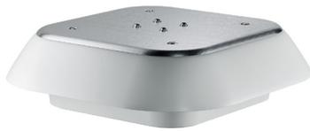
TP series roof exhaust units represent an optimal solution for heat dissipation through the top of electrical cabinets. They are ideal for indoor use where there is limited space on the front and side panels. According to the ambient conditions these units can be operated with fan (forced air) or without a fan (natural air convection).
