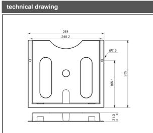
An handy accessory for documentation, this holder in PC/ABS alloy can be easily applied on the enclosure door through a tape.
