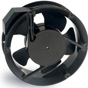
Axial fans provide forced-air cooling solution to temperature-sensitive applications. Compact fans with AC shaded pole or capacitor and DC brushless motor are designed for ventilation and spot cooling of internal machinery components, especially in areas in confined spaces. Available also versions tested to withstand harsh environmental conditions (IP55, IP68, all metal and HTR fans).
