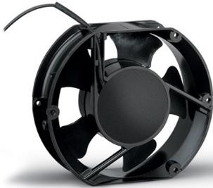
Axial fans provide forced-air cooling solution to temperature-sensitive applications. Compact fans with AC shaded pole or capacitor and DC brushless motor are designed for ventilation and spot cooling of internal machinery components, especially in areas in confined spaces. Available also versions tested to withstand harsh environmental conditions (IP55, IP68, all metal and HTR fans).
