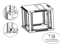
[5] use the M5\*10 self-tapping lock screw to install the rails, the screw from outside to inside
