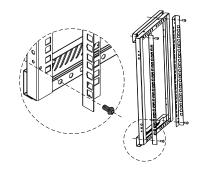
Fix 19" mounting rails to the first holes of top & bottom of side frames by 8 pcs of M5X10 screws.
