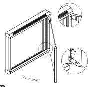
Open the front door by key, pull the door latch downward, refer to the picture, remove the front door from front frame, put them separate for the preparation of the frame assembly.
