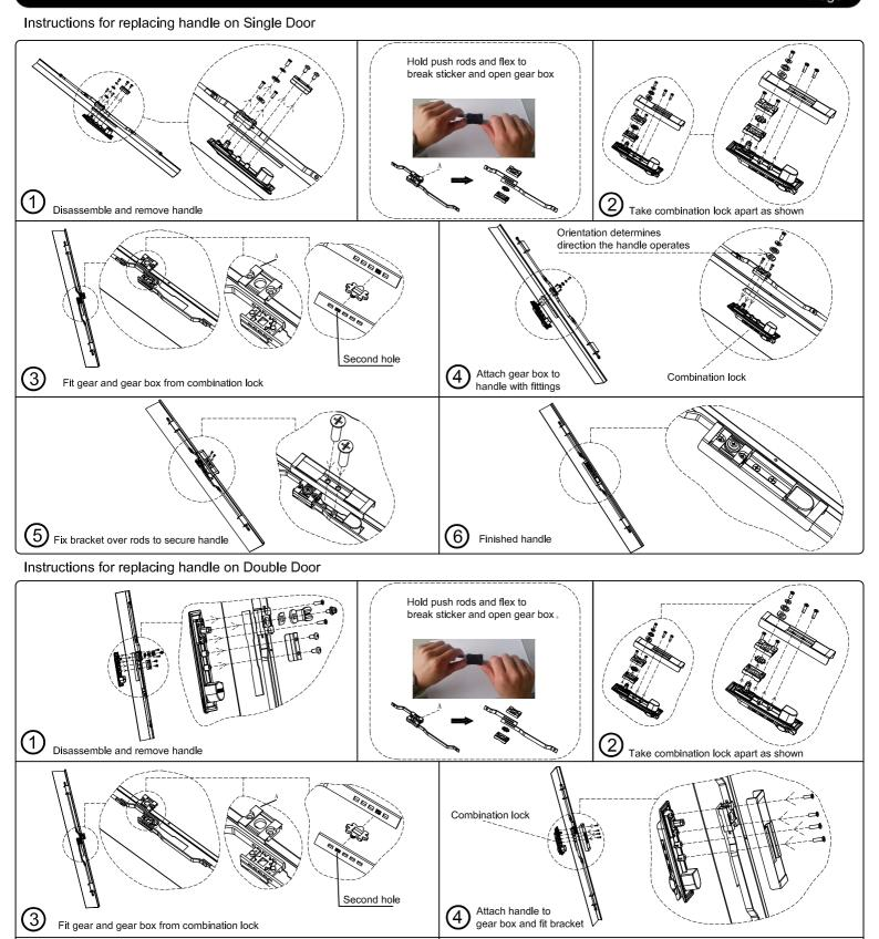
Orientation determines direction the handle operates.
