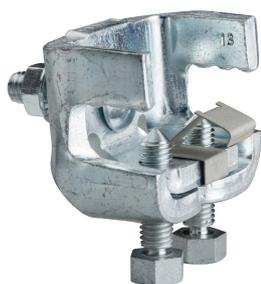
This code-compliant Structural Attachment is part of the nVent CADDY line of innovative rigid bracing system, designed to provide superior performance and meet the highest seismic load requirements. Its innovative design allows quick and easy installation onto both top or bottom flange of a wide range of steel I-Beams. Its snap-off bolts make inspection of seismic sway braces simple.
