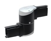
Syspend 281-Max Intermediate Joint to join two horizontal tubes together for a longer run. Arm can be rotated or turned 300 degrees. Includes safety stop and maintenance-free bearing. Use of the Intermediate Joint reduces the system load capacity to 179 lb. (81.2 kg) at 3.3 ft. (1 m).
