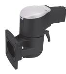
Syspend 180-Max Horizontal Panel Coupling mounts a horizontal tube to the back of an enclosure or screen using Video Electronics Standards Association (VESA) mounting. The coupling has mounting holes drilled for standard VESA 75 and 100 flange sizes. It enables the enclosure to rotate 300 degrees and can be locked into a given position. The horizontal panel coupling has a safety stop and maintenancefree bearings.
