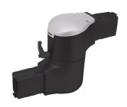
Syspend 180-Max Intermediate Joint joins two horizontal tubes together for a longer length. The arm can be rotated 300 degrees. Includes safety stop and maintenance-free bearings. Use of the intermediate joint reduces the system load rating capacity to 146 lb. (66 kg) at 3.3 ft. (1 m).
