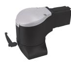
Syspend 180-Max Flange Elbow Coupling attaches directly to the enclosure for applications where a vertical tube is not required. It enables the enclosure to rotate 300 degrees and can be locked into a given position. The flange elbow coupling has a safety stop and maintenance-free bearings.
