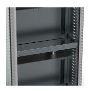
The galvanised steel compartment, MSCP, allows for plug-in connections with the busbar and can be pulled out from the enclosure without having to turn the power off. Maintenance can then be performed without losing power to the other parts of the enclosures, which will eliminate unnecessary downtime.
