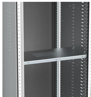
The galvanised steel shelf, MSCC, covers a partial depth of an enclosure and is ideal for equipment requiring strong fixation, such as heavy air circuit breakers. It leaves the rear of the enclosure accessible for easy installation and wiring.
