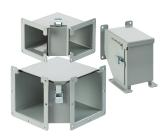
Lay-in Hinged-Cover 90-Degree Elbows are used for rightangle wireway installations. Because sections of lay-in wireway can be mounted with covers oriented in any direction, three different 90-degree elbows are available. Proper selection allows the user to maintain the same access and thereby preserve the lay-in feature for right-angle installations.
