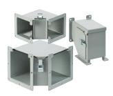
Lay-in Hinged-Cover 90-Degree Elbows are used for rightangle wireway installations. Because sections of lay-in wireway can be mounted with covers oriented in any direction, three different 90-degree elbows are available. Proper selection allows the user to maintain the same access and thereby preserve the lay-in feature for right-angle installations.
