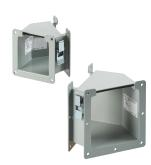
Lay-in Hinged-Cover 45-Degree Elbows are used for continuous wireway runs with 45-degree turns. Because sections of lay-in wireway can be mounted with covers oriented in any direction, three different 45-degree elbows are available. Proper selection allows the user to maintain the same access and thereby preserve the lay-in feature for right-angle installations.
