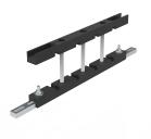
This busbar support, ECBS, is available for one or two bars up to  $80 \times 5$  mm or one bar up to  $80 \times 10$  mm. The support can be mounted both horizontally and vertically. It is available off the shelf and tested according to IEC 61439.
