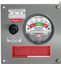
Small-Volume Purging/Pressurization Systems are an alternative to NEMA Type 7 or 9 enclosures. The C1 model allows general-purpose enclosures, up to two cubic feet, to be used in certain Class 1 hazardous locations. The C2 model allows general purpose enclosures, up to 10 cubic feet, to be used in certain Class 2 hazardous locations.
