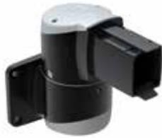
Horizontal Wall Joint mounts suspension system to vertical surface, allowing tube to extend horizontally. Arm can be rotated or turned 300 degrees. Includes safety stop and maintenance-free bearing. RAL 9005 black finish. Die-cast aluminum construction. Includes two removable cable access covers, installation instructions, gaskets and tube setscrews. Surface mounting hardware not provided.
