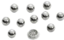
Rotation limiters can be retro-fit on coupling and joint components and are adjustable in increments of 13.7 degrees. Limits rotation of couplings and joints which normally rotate 300 degrees. Kit includes ten steel balls, plug and installation instructions.
