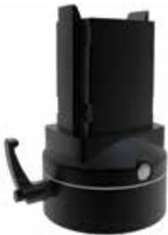
Flange Coupling attaches a tube to the enclosure, enabling 300-degree enclosure rotation. Enclosure can be locked in position. Flange Coupling has safety stop and maintenance-free bearing. RAL 9005 black finish. Die-cast aluminum construction. Includes installation instructions, gaskets, tube setscrews and enclosure mounting hardware.
