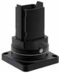
Rotary Base allows the entire suspension system to rotate at the point of attachment on a horizontal surface. Arm can be rotated or turned 300 degrees. Includes safety stop and maintenance-free bearing. RAL 9005 black finish. Die-cast aluminum construction. Includes installation instructions, gaskets and tube setscrews. Surface mounting hardware not provided.
