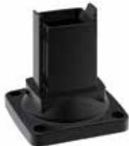
Wall Flange allows for fixed positioning on a horizontal or vertical surface when rotation is not needed. RAL 9005 black finish. Die-cast aluminum construction. Includes installation instructions, gaskets and tube setscrews. Surface mounting hardware not provided.
