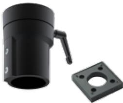
Use Flange Coupling to attach the Vertical Motion Pedestal Tube to the enclosure. Enclosure can be rotated 300 degrees and locked in position. Includes safety stop and maintenance-free bearing. RAL 9005 black finish. Die-cast aluminum construction. Includes installation instructions, gaskets and enclosure mounting hardware.
