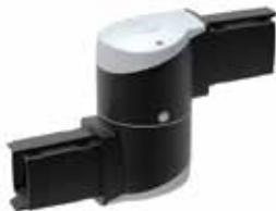
Use Intermediate Joint to join two horizontal tubes together for a longer run. Arm can be rotated or turned 300 degrees. Includes safety stop and maintenance-free bearing. RAL 9005 black finish. Die-cast aluminum construction. Includes two removable cable access covers, installation instructions, gaskets and tube setscrews.
