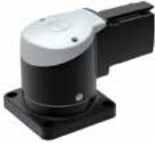
Set-Up Joint mounts suspension system to a horizontal surface. Arm can be rotated or turned 300 degrees. Includes safety stop and maintenance-free bearing. RAL 9005 black finish. Die-cast aluminum construction. Includes removable cable access cover, installation instructions, gaskets and tube setscrews. Surface mounting hardware not provided.
