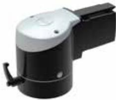
Flange Elbow Coupling attaches directly to the enclosure for applications where a vertical tube is not required. Enables enclosure to be rotated 300 degrees and locked in position. Includes safety stop and maintenance-free bearing. RAL 9005 black finish. Die-cast aluminum construction. Includes cable access cover, installation instructions, gaskets, tube setscrews and enclosure mounting hardware.
