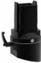
Use Angled Coupling Tilted Backward to mount enclosure at a 15-degree backward angle. Enclosure can be rotated 300 degrees and locked in position. Includes safety stop and maintenance-free bearing. RAL 9005 black finish. Die-cast aluminum construction. Includes installation instructions, gaskets, tube setscrews and enclosure mounting hardware.
