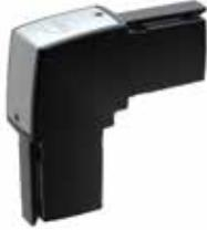
Elbow provides a 90-degree bend in the suspension system. RAL 9005 black finish. Die-cast aluminum construction. Includes removable cable access cover, installation instructions, gaskets and tube setscrews.
