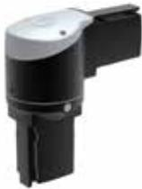
Rotatable elbow provides a 90-degree bend in the suspension system and allows the vertical tube to rotate 300 degrees. Includes safety stop and maintenance-free bearing. RAL 9005 black finish. Die-cast aluminum construction. Includes removable cable access cover, installation instructions, gaskets and tube setscrews.
