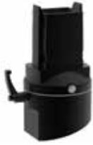
Use Angled Coupling Tilted Forward to mount enclosure at a 15-degree forward angle. Enclosure can be rotated 300 degrees and locked in position. Includes safety stop and maintenance-free bearing. RAL 9005 black finish. Die-cast aluminum construction. Includes installation instructions, gaskets, tube setscrews and enclosure mounting hardware.
