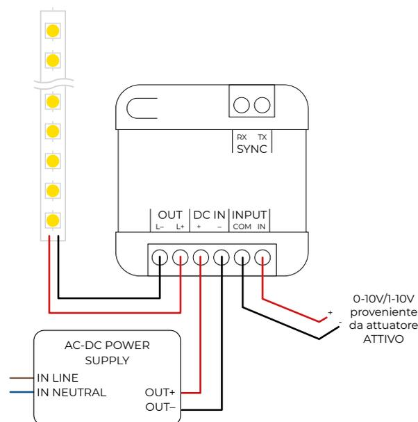
FIG. 3 - collegamento 0-10V/1-10V 13/22160-00
