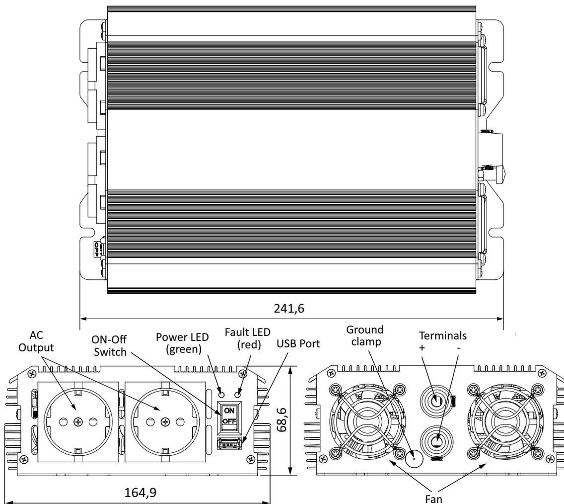
**CAUTION:** Do not reverse. Use red battery cord to connect (+) of a battery to (+) terminal and then, use black battery cord to connect (-) battery to (-) terminal.
