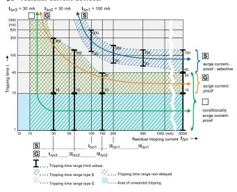
**IEC 60364-4-41** deals with additional protection: The use of RCDs with a rated residual operating current not exceeding 30 mA, is recognized in a.c. systems as additional protection in the event of failure of the provision for basic protection and/or the provision for fault protection or carelessness by users.
