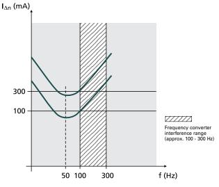
This sample tripping characteristic of a 100 mA RCD and a 300 mA RCD shows the following: In the frequency range around 50 Hz, the RCDs trip as required (50 - 100 % of the indicated  $I_{\Delta n} \rangle$ .
