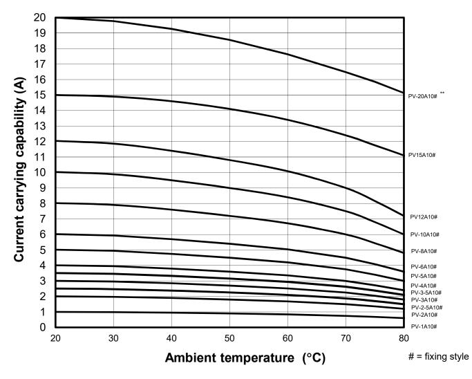
No additional derating is required for PV fuse links installed in ganged modular fuse holders without spacing between units, provided that the rating used is  $>1.56 \times I_{\infty}$ .
