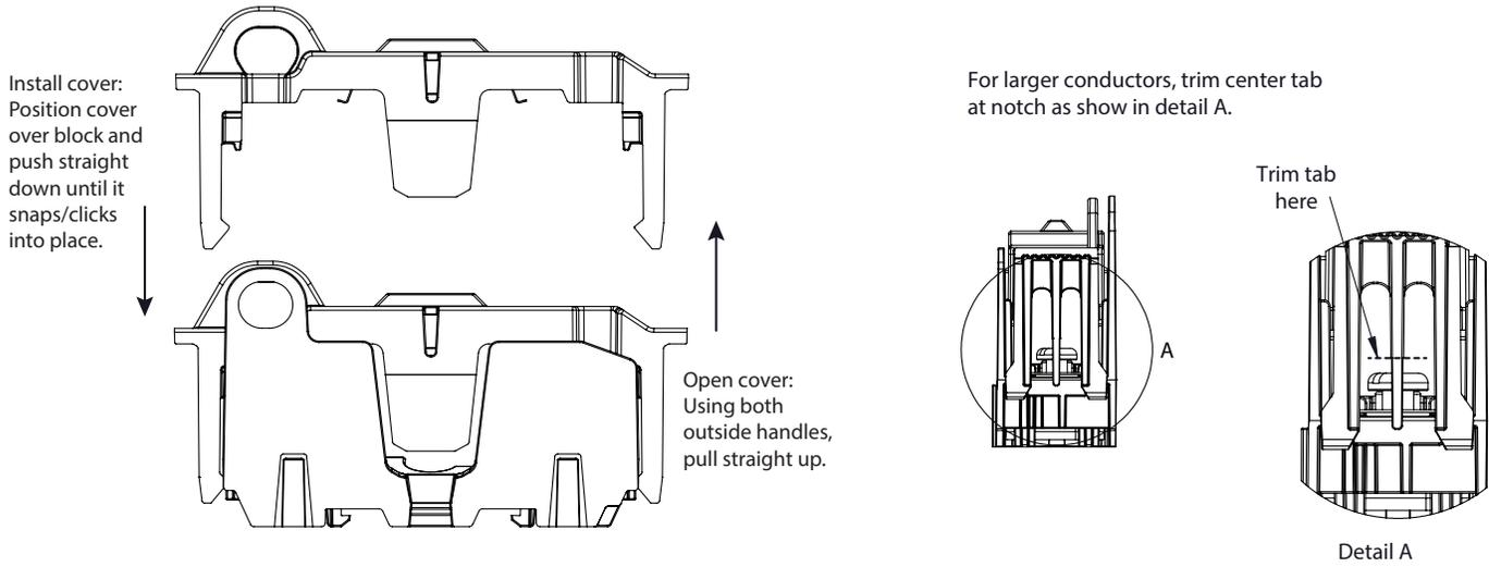
**Installing blocks on DIN-Rail**
