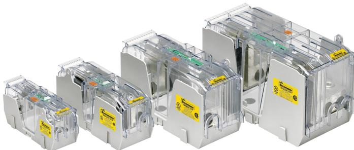
100 to 600 amp knifeblade fuse blocks are panel mount with multiple holes for installation flexibility and the modular design allows blocks to snap together for the desired number of poles. They accept optional snap-on covers for IP20 finger-safe protection and feature a lockout/tagout provision to improve electrical safety.
