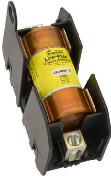
30 and 60 amp ferrule fuse blocks have DIN-rail and panel mounting capability, the modular designs allows blocks to snap together for the desired number of poles. They accept optional snap-on covers for IP20 finger-safe protection and feature a lockout/tagout to improve electrical safety.
