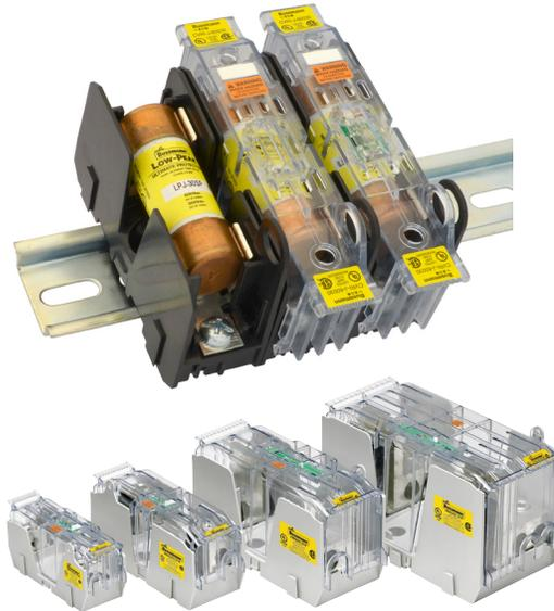
Knifeblade fuse blocks from 100 to 600 amps feature phase barriers between poles for additional safety with up to four mounting holes per pole increase installation flexibility. All knifeblade blocks meet UL creep and clearance requirements for Industrial Power Circuits (UL 508 and UL 845).
