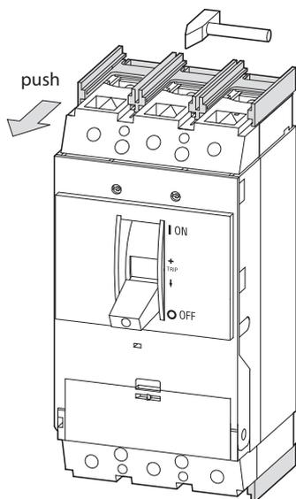
The barrier (shown shaded in the diagrams) is held tightly into grooves on top and bottom sides of the breaker or switch and must be removed in order to mount ...-XKA... Mechanical (Tunnel) lug connectors on NZM2 and NZM3 Circuit-Breakers and switches. To remove: From the back of the device, use an appropriate tool to gently tap each side of the barrier to help slide it out.
