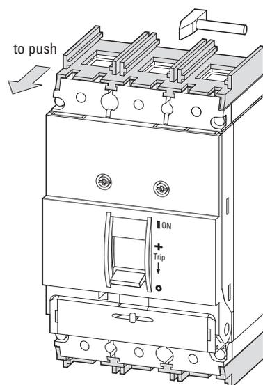
The barrier (shown shaded in the diagrams) is held tightly into grooves on top and bottom sides of the breaker or switch and must be removed in order to mount NZM1-XKA and -XKS connectors.
