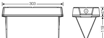
Prepare the required cable entry and fit a cable gland. Fix the gallery to the ceiling or wall using the stainless steel screws (included).
