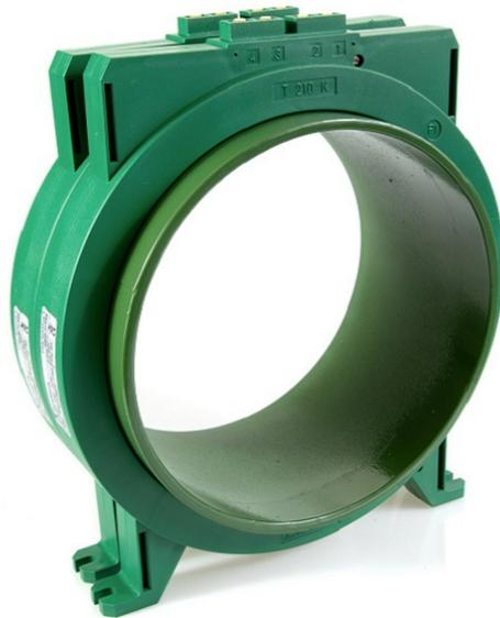
In large systems, when busbars are used or there are many cables, it may happen that the active conductors cannot be centered and that they pass near to the internal casing of the toroidal current transducer. This does not represent a correct installation as, in the event of high peaks or high load currents, it is possible to run into an incorrect reading of the residual current and consequently in untimely trips.
