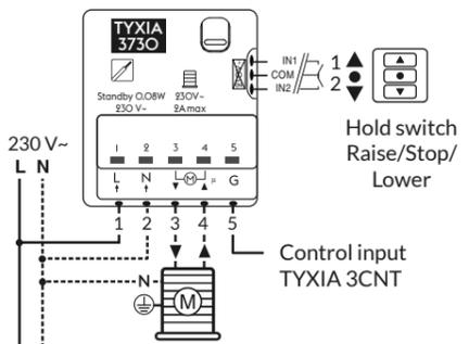
**Switch off the system before performing any action on the receiver.**
