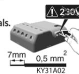
**Do not strip the wires when they are connected to the product as you could damage the internal connector.**
