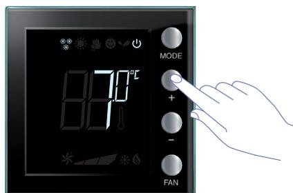
The current set-point flashes for a few seconds. During this time press + or – to change the temperature. The display flashes for 4 seconds, showing the new set-point.
