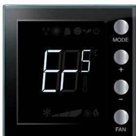
(\*) **NOTE:** if ER4 or a temperature very different from the one felt are displayed, or after the first installation, wait at least 5 hours before checking the operation again, or carrying out the calibration procedure.
