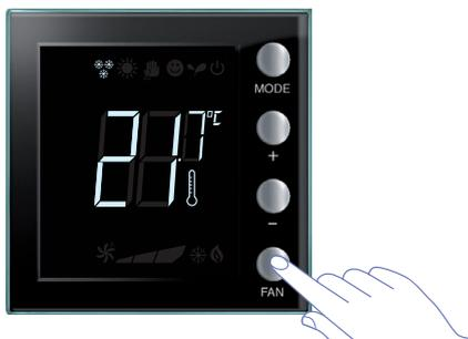
The display brightness can be adjusted on 10 levels.
