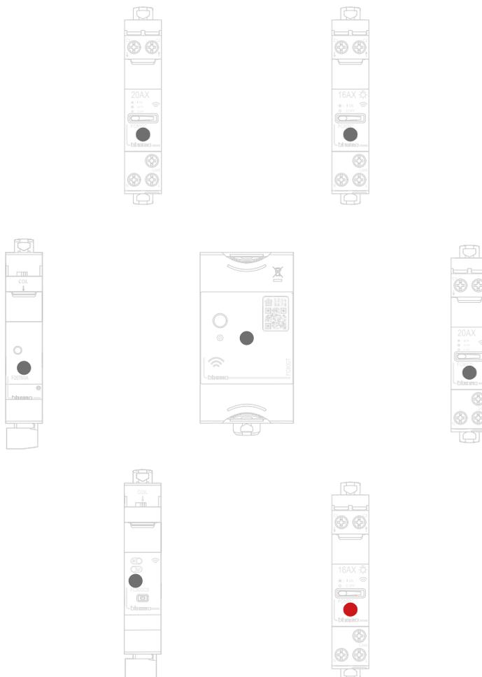
Check that the LEDs of all the devices are off, with the exception of the device to add, which must have a steady red LED.
