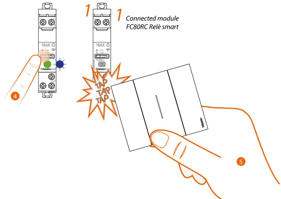
4. Press and hold down the control pushbutton until the LED flashes blue then release.
