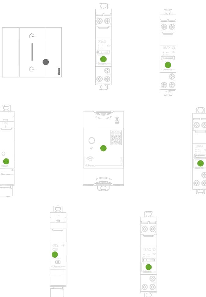
Check that the LEDs of all the devices immediately turn green steady (with the exception of the wireless LEDs, which will be off).
