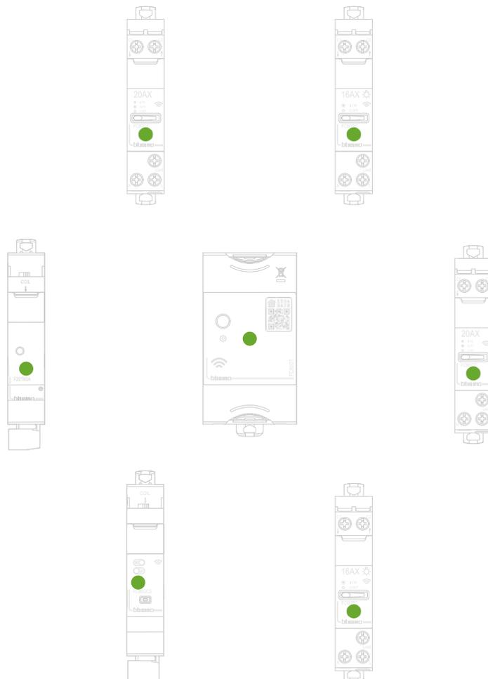
Check that the LEDs of all the devices turn green steady.
