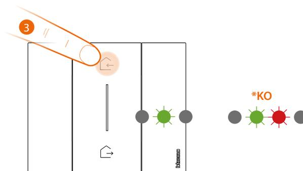
3. Press and release one of the control keys: the LED flashes green; release it and wait for the LED to turn off.
