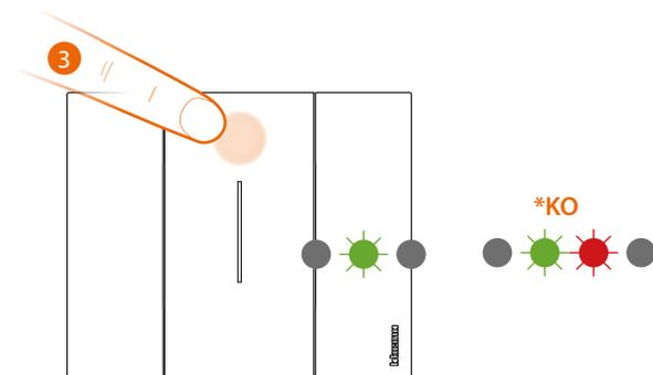
3. Press and release one of the two control keys: the LED flashes green; wait until it turns off. The control is now associated to your Smart electric system. Let's now continue with the association of the light to the control.
