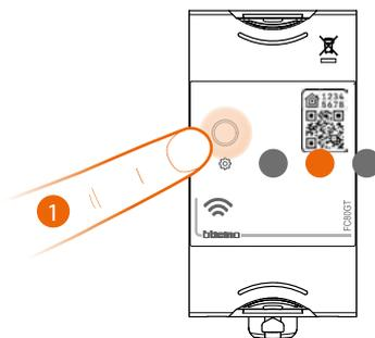
1. press and hold down the reset pushbutton, the LED turns orange.
