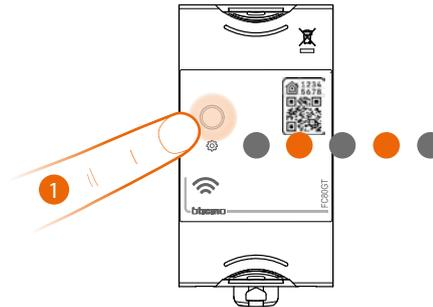
1. Press and hold down the reset pushbutton, the LED turns orange then switches off and at last turns orange again.
