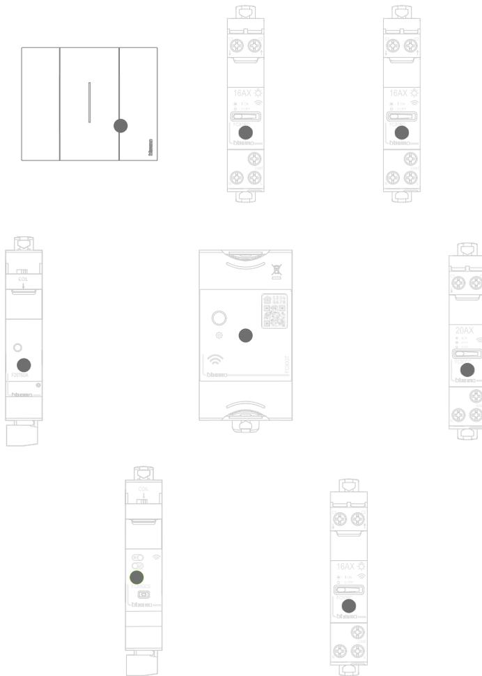
Check that the LEDs of all the devices immediately turn off: the wired devices are now associated with each other.
