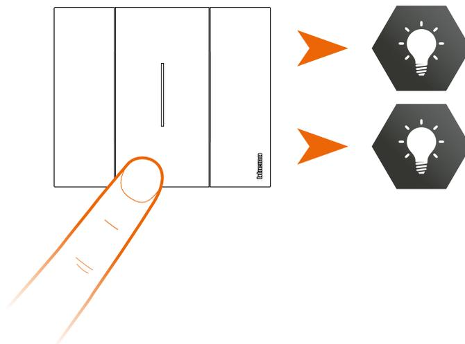
After associating the wireless light control to the smart relays, it is possible to activate the connected loads.
