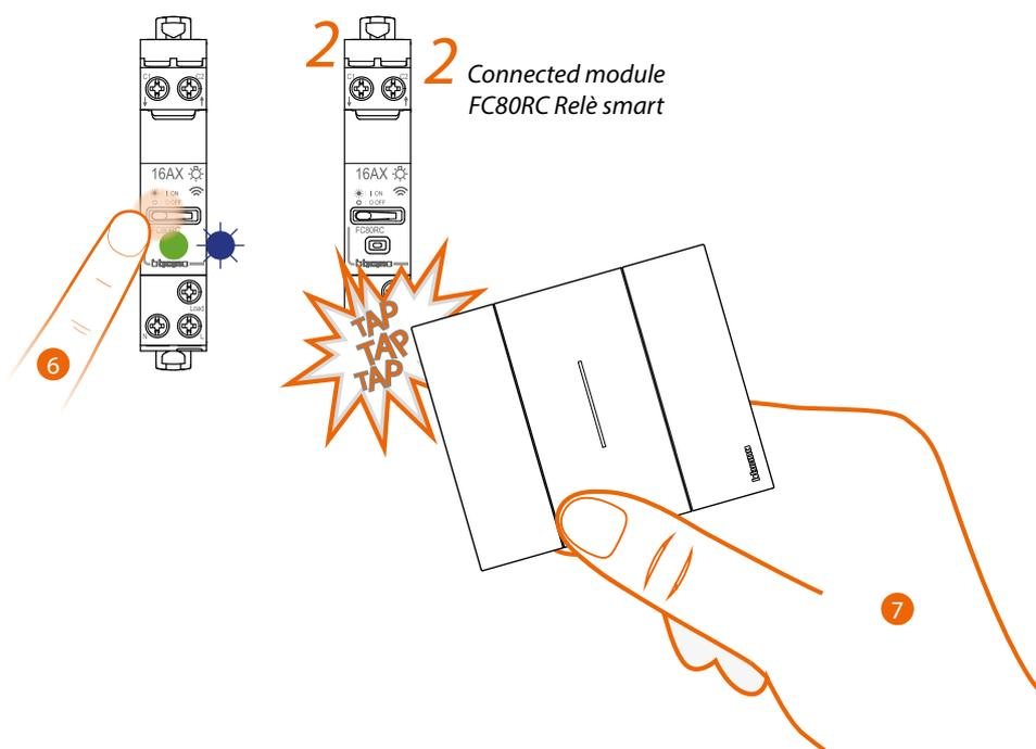
6. Press and hold down the control pushbutton until the LED flashes blue then release.
