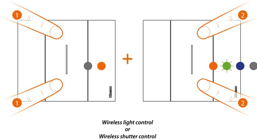
1. Press at the same time the two pushbuttons of the control to dissociate until the LED turns orange.
