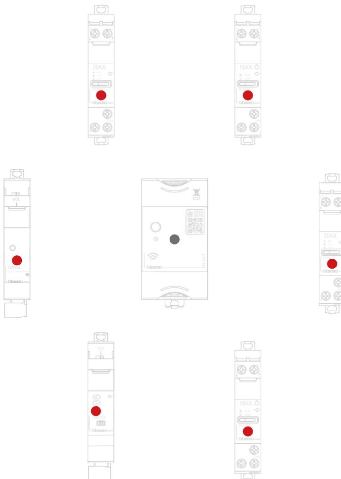
Check that the LEDs of all the devices turn on red steady (with the exception of the gateway LED, which remains off).
